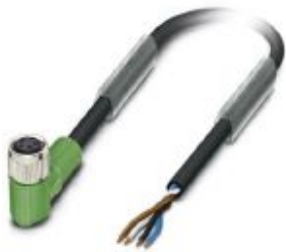
Sensor/actuator cable, 4-position, PUR halogen-free, black-gray RAL 7021, free cable end, on Socket angled M8, cable length: 20 m
