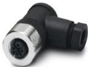
Connector, 4-position, Socket angled M12, Coding: A, Screw connection, knurl material: Stainless steel 1.4404, cable gland Pg7, external cable diameter 4 mm ... 6 mm
