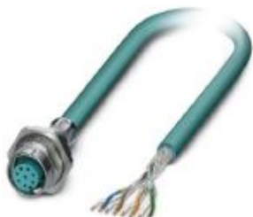
Bus system flush-type socket, Ethernet, 8-pos., M12, shielded, rear/screw mounting with M16 thread, with 2 m bus cable, 4 x 2 x 0.14 mm 2
