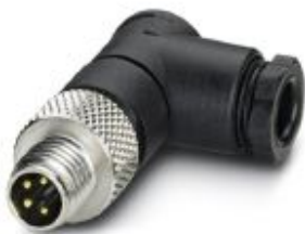
Connector, Universal, 4-position, Plug angled M8, Coding: A, Solder connection, knurl material: Nickel-plated brass, external cable diameter 3.5 mm ... 5 mm
