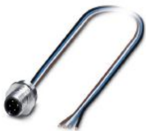
Sensor/actuator flush-type plug, 4-pos., M12, A-coded, front/screw mounting with Pg9 thread, with 0.5 m TPE litz wire, 4 x 0.34 mm 2 , stainless steel version
