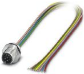
Sensor/actuator flush-type plug, 8-pos., M12, front/screw mounting with Pg9 thread, with 0.5 m TPE litz wire, 8 x 0.25 mm 2 , stainless steel version
