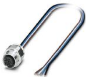
Sensor/actuator flush-type socket, 4-pos., M12, A-coded, front/screw mounting with Pg9 thread, can be positioned, with 0.5 m TPE litz wire, 4 x 0.34 mm 2 , stainless steel version
