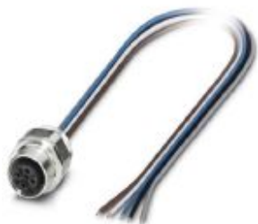
Sensor/actuator flush-type socket, 5-pos., M12, A-coded, front/screw mounting with Pg9 thread, can be positioned, with 0.5 m TPE litz wire, 5 x 0.34 mm 2 , stainless steel version
