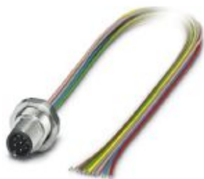
Sensor/actuator flush-type plug, 8-pos., M12, rear/screw mounting with Pg9 thread, with 0.5 m TPE litz wire, 8 x 0.25 mm 2 , high-grade steel version
