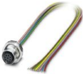
Sensor/Actuator flush-type socket, 8-pos., M12, A-coded, rear/screw mounting with Pg9 thread, with 0.5 m TPE litz wire, 8 x 0.25 mm 2 , on high-grade steel version
