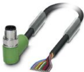
Sensor/actuator cable, 12-position, PVC, black RAL 9005, Plug angled M12 SPEEDCON, coding: A, on free cable end, cable length: 10 m
