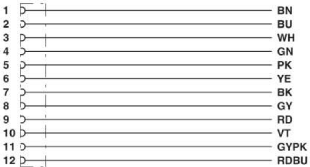
Contact assignment of the M12 socket
