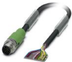
Sensor/actuator cable, 17-position, PVC, black RAL 9005, Plug straight M12 SPEEDCON, coding: A, on free cable end, cable length: 10 m
