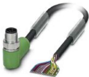
Sensor/actuator cable, 17-position, PVC, black RAL 9005, Plug angled M12 SPEEDCON, coding: A, on free cable end, cable length: 5 m
