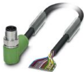
Sensor/actuator cable, 17-position, PVC, black RAL 9005, Plug angled M12 SPEEDCON, coding: A, on free cable end, cable length: 10 m
