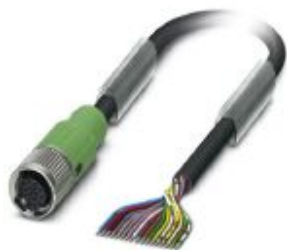
Sensor/actuator cable, 17-position, PVC, black RAL 9005, free cable end, on Socket straight M12 SPEEDCON, coding: A, cable length: 5 m
