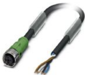
Sensor/actuator cable, 4-position, PUR, black-gray RAL 7021, free cable end, on Socket straight M12 SPEEDCON, coding: A, cable length: 10 m
