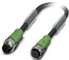
Sensor/actuator cable, 4-position, PUR, black-gray RAL 7021, Plug straight M12 SPEEDCON, coding: A, on Socket straight M12 SPEEDCON, coding: A, cable length: 1 m
