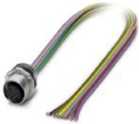
Sensor/actuator flush-type socket, 12-pos., M12 SPEEDCON, front/screw mounting with M16 thread, with 0.5 m PVC litz wire, 12 x 0.14 mm 2
