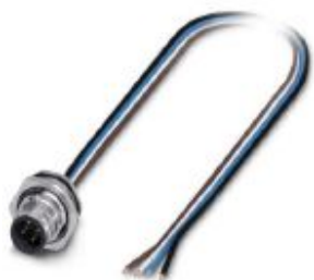
Sensor/actuator flush-type plug, 4-pos., M12 SPEEDCON, rear/screw mounting with Pg9 thread, with 0.5 m TPE litz wire, 4 x 0.34 mm 2
