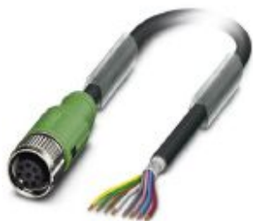
Sensor/actuator cable, 8-position, PUR halogen-free, black-gray RAL 7021, shielded, free cable end, on Socket straight M12 SPEEDCON, coding: A, cable length: 3 m
