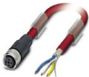
Bus system cable, CC link (10 Mbps), 4-position, PVC, red, shielded, free cable end, on Socket straight M12, coding: A, cable length: 5 m
