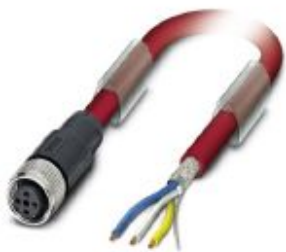
Bus system cable, CC link (10 Mbps), 4-position, PVC, red, shielded, free cable end, on Socket straight M12, coding: A, cable length: 10 m
