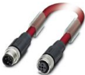
Bus system cable, CC link (10 Mbps), 4-position, PVC, red, shielded, Plug straight M12, coding: A, on Socket straight M12, coding: A, cable length: 15 m
