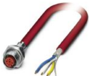
Bus system flush-type socket, CC-Link, 4-pos., M12, shielded, rear/screw mounting with M16 thread, with 5 m bus cable
