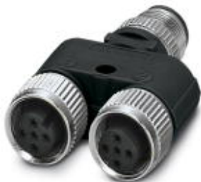
Y distributor, 5-position, unshielded, Plug straight M12, A-coded, on Socket straight M12, A-coded and Socket straight M12, A-coded, Parallel distributor
