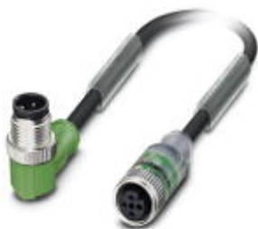
Sensor/actuator cable, 4-position, PUR halogen-free, black-gray RAL 7021, Plug angled M12, A-coded, on Socket straight M12, A-coded, with 3 LEDs, cable length: 4 m
