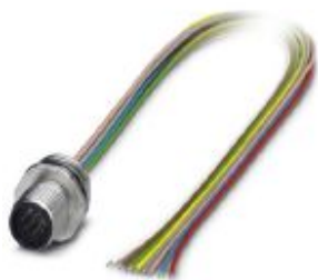
Sensor/actuator flush-type plug, 8-pos., M12, A-coded, front/screw mounting with M16 thread, with 0.1 m TPE litz wire, 8 x 0.14 mm 2
