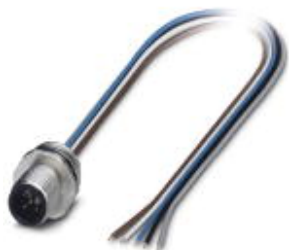
Sensor/Actuator flush-type plug, 5-pos., M12, A-coded, front/screw mounting with Pg9 thread, with 0.115 m TPE litz wire, 5 x 0.34 mm 2
