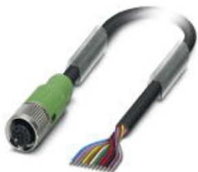
Sensor/actuator cable, 12-position, PVC, black RAL 9005, free cable end, on Socket straight M12 SPEEDCON, A-coded, cable length: 15 m
