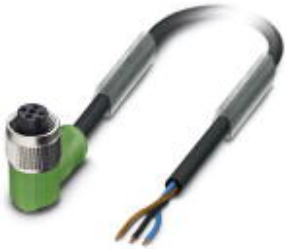
Sensor/actuator cable, 3-position, PUR halogen-free, black-gray RAL 7021, free cable end, on Socket angled M12, A-coded, cable length: 20 m
