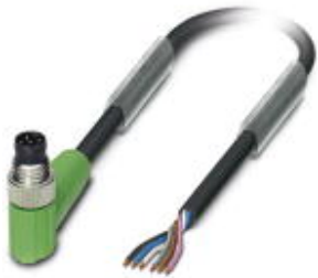
Sensor/actuator cable, 6-position, PUR halogen-free, black-gray RAL 7021, Plug angled M8, on Plug angled M8, cable length: 10 m
