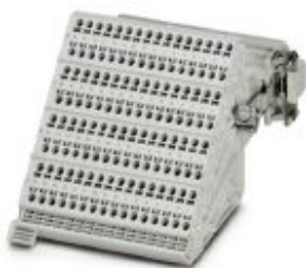
HEAVYCON terminal adapter male insert, D64 series, 64-pos., right PE connection for the left side of the control cabinet, push-in connection
