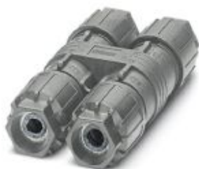
H distributor, QUICKON connection, number of positions: 4, 1 mm 2 ... 2.5 mm 2 , 690 V, 20 A, gray, with QUICKON nut, cable diameter range: 6 mm ... 10 mm
