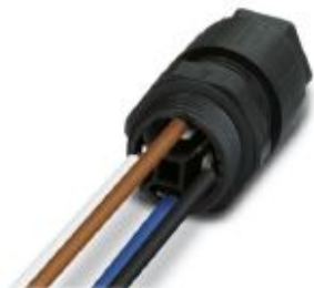
Panel feed-through, with wire output 1.5 mm 2 and 0.5 m litz wire: connecting thread: M20x1.5, 4-pos., black
