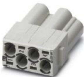
HEAVYCON contact insert module, shock-proof pins, 4-pos. to 40 A, crimp connection
