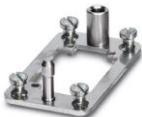
Docking frames for racks, for type B6 contact inserts, with 4 M5 flat headed screws, slide-in offset for x/y axis of ±1.5 mm
