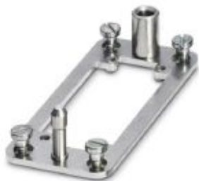
Docking frame for racks, for contact inserts of B16 type, with four M5 flat headed screws, rack balance x/y axis +/- 1.5 mm
