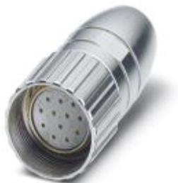
Cable connector, straight, shielded: yes, Screw locking, M23, No. of pos.: 12, type of contact: Socket, Crimp connection
