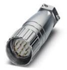
Cable connector, with Pg11 connection thread, straight, shielded: yes, Screw locking, M23, No. of pos.: 17, type of contact: Pin, Crimp connection, cable diameter range: 7.5 mm ... 9.5 mm
