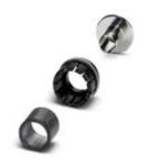
Cable clamp type cage and shield adapter, shielded: yes, litz wire bundle diameter: 6.2 mm, cable diameter range: 7.5 mm ... 9.5 mm
