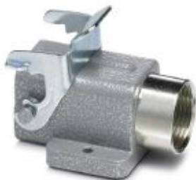
HEAVYCON D7 box mounting base, with single locking latch, height 25.5 mm, with 1 x M20 gland, with open bottom, zinc
