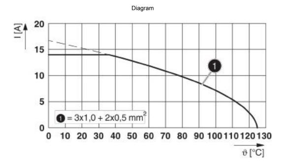
I = current strength, ϑ = ambient temperature, 3x 14 A + 2x 2 A constant
