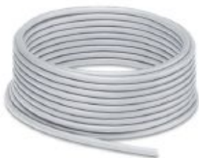
PROFINET power cable, 5x 2.5 mm 2 , stranded (7-wire), outer sheath: PVC, outside diameter 11.8 mm, RAL 7001 (silver gray), oil-resistant, cable ring: 100 m
