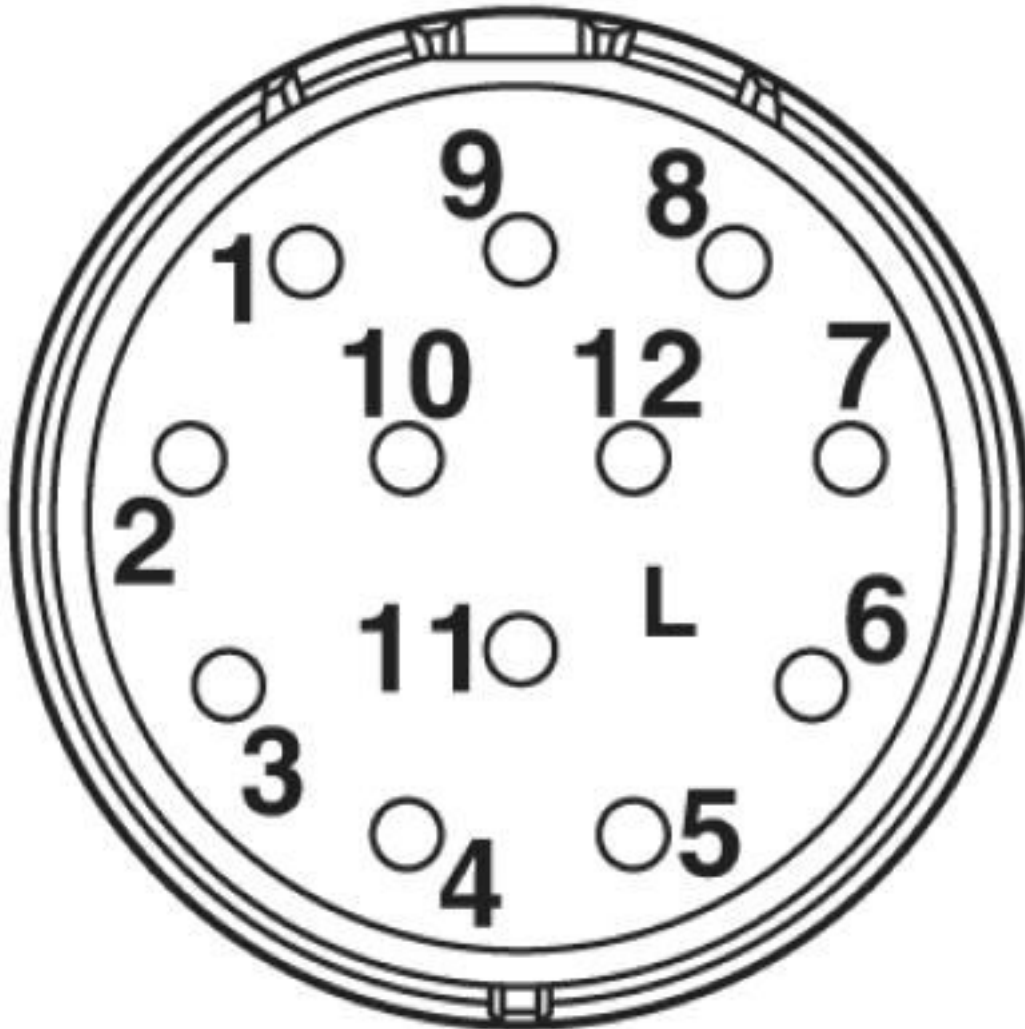
Contact chamber numbering (view of plug-in side), standard socket
