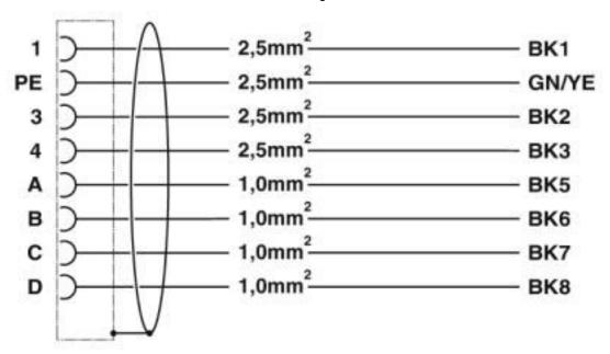
Contact assignment of M23 plugs/sockets
