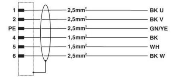
Contact assignment of M23 plugs/sockets
