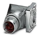
Device connector, front mounting, angled rotatable, for standard and SPEEDCON interlock, M17, number of positions: 8, type of contact: Socket, Axial O-ring, 4x Ø2,7, shielded: yes, flange dimensions: 25.75 mm, very connection method: Crimp connection
