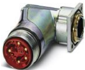
Device connector for front wall, SB, angled rotatable, shielded: yes, for standard and SPEEDCON interlock, M40, No. of pos.: 4+4+4+PE, type of contact: Pin, Crimp connection, Axial O-ring, 4x Ø4,2
