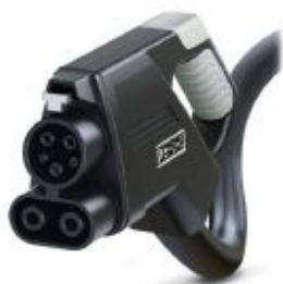
, DC charging cable with vehicle connector, open cable end, CCS type 1, Combined Charging System, SAE J1772, IEC 62196-3, 60 A / 600 V (DC), cable: 5 m, black, straight
